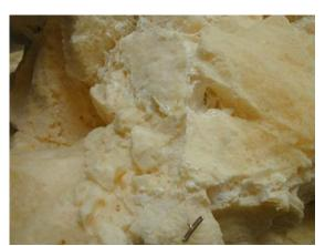
Let cure 1 hour and 3 hours, depending on moisture in the air. Tear off risen foam flush with edges, foam must cure to a point of not rising anymore but not be fully cured. You want to expose the rough texture of the inner foam.
